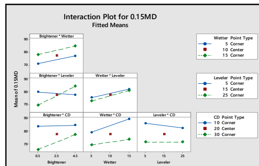
Figure 5 - Interaction Plot for 0.15 mm diameter TH in 0.8 mm panel, Aspect Ratio = 5.3
