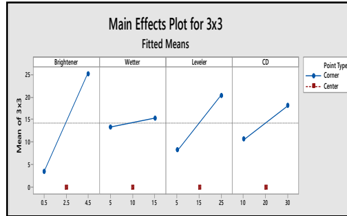
Figure 6 - Main Effect Plot, 3x3 (75 μm X 75 μm) Via dimple as a function of Brightener, Wetter, Leveler and CD
