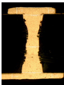
X-Via Filling Void-Free
